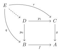
and call the square a pullback diagram,  $p_0$  a pullback of g along f and  $p_1$  a pullback of f along g. The pullback is also called the fiber product as it is actually the product in the category of fibrations over A. Sometimes, the object D itself is loosely called the pullback and it is denoted by  $B \times_A C$ .
